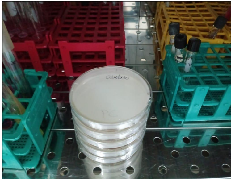
Incubar 48 \pm 2 h a 35^\circ\text{C}
